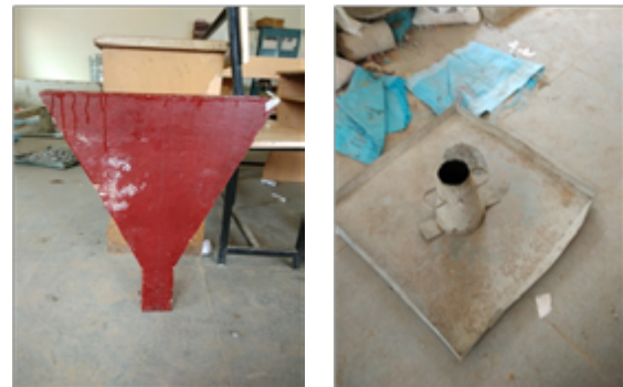
Figure 2: V-Funnel and Slump Flow Apparatus.
