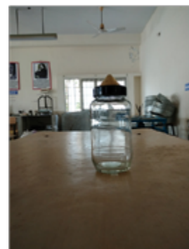
Figure 1: Pycnometer used for finding out Specific Gravity of materials.
